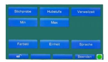
**Sample** = number of measuring points to be measured (with automatic measurement)
