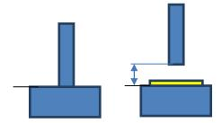
**Dwell time** = how long the measuring sensor should dwell on the object to be measured until the measured value is recorded. (the correct values are stored in the corresponding standards).
